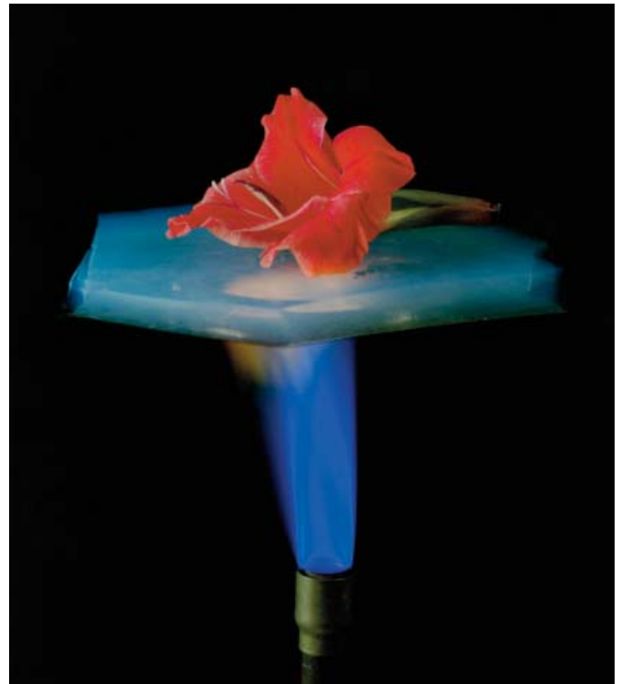
Invented in 1931 by Dr Samuel Kistler at the College of the Pacific in California, aerogels are around 97% air in small nanopores.
